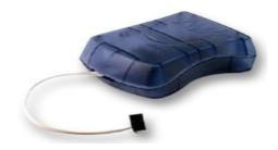
Connect your Programmer's 6 pin socket to the ISP header on the board. Pin 1 on the ISP header is usually marked with a small triangle. Then connect the a 5V DC power source to the PCB pins.
